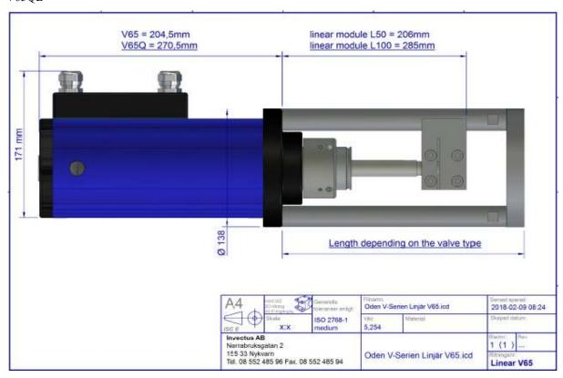
V30Q/V65Q (Q=quick, actuator with servo motor V30QL/V65QL (L= with linear module)
