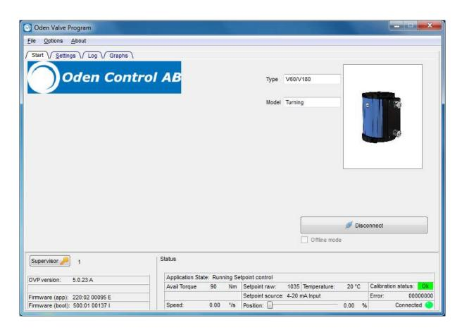
THE ODEN VALVE PROGRAM, OVP, CAN BE USED TO CHANGE THE DEFAULT SETTINGS OF TORQUE, SPEED, WORKING RANGE ETC. HOWEVER, IT IS NOT REQUIRED FOR OPERATING THE ACTUATOR. IF THE DEFAULT VALUES ARE ADEQUATE FOR YOUR APPLICATION, IT IS NOT NECESSARY TO USE THE SOFTWARE. A LIST OF DEFAULT VALUES CAN BE DOWNLOADED FROM OUR WEBSITE.
