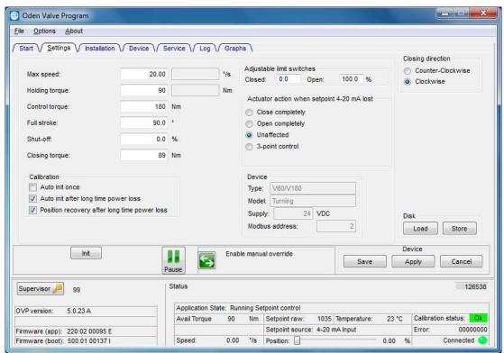
Check Firmware (app) and Firmware (boot) are visible, when using V5.0.23A program.
